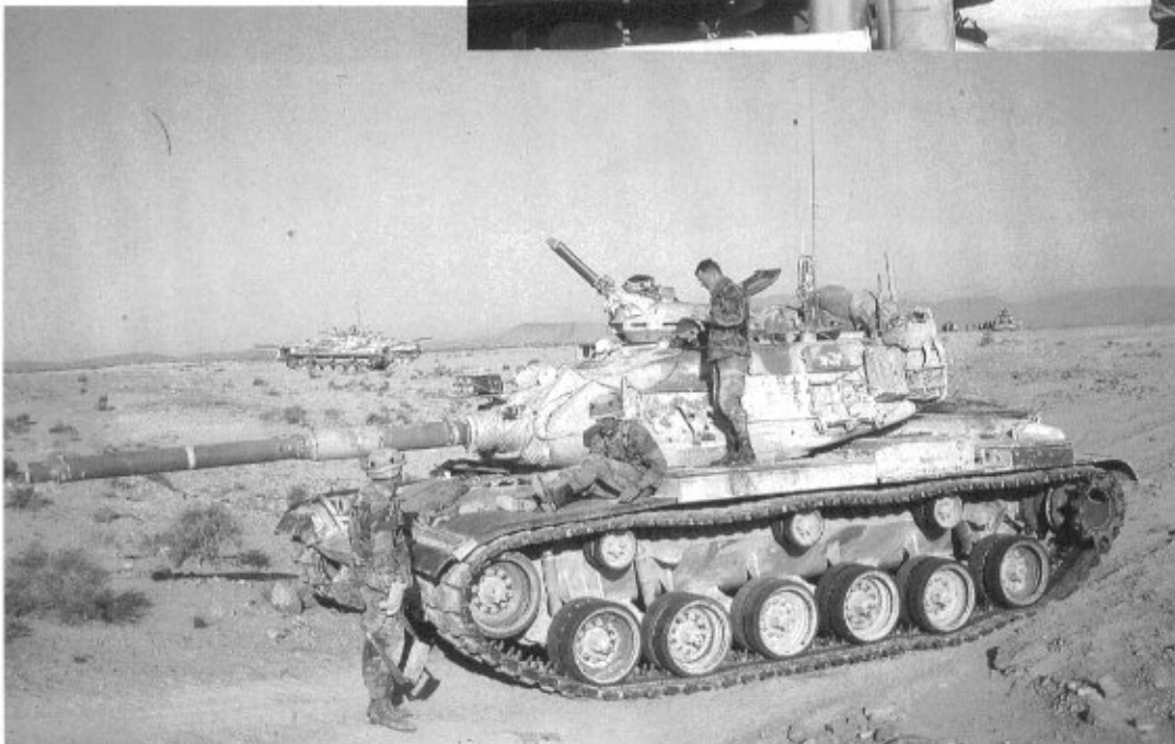
In addition to the 105mm main gun, the M60A3 tank is equipped with a Belgian designed M240 7.62mm coaxial machine gun and a M85 .50 caliber machine gun fitted on the commander's cupola for use against troops and lightly armored vehicles. (Greg Stewart Photo)
