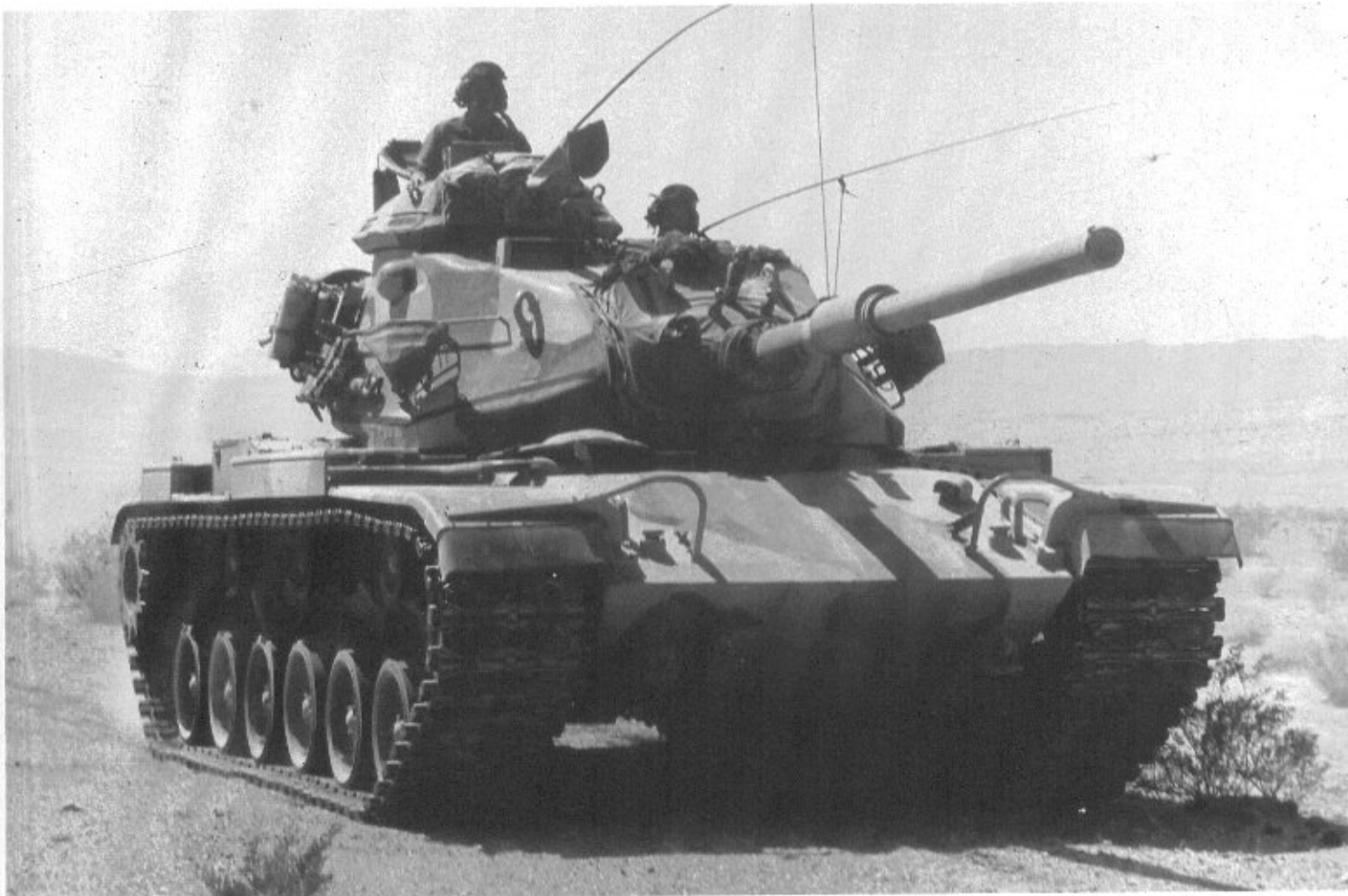
The gun elevating and turret traversing system consists of mechanical, electrical, and hydraulic components so arranged as to permit either the gunner or commander to traverse the turret 360 degrees in either direction or to depress and elevate the 105mm gun cannon. (U.S. Army Photo)
