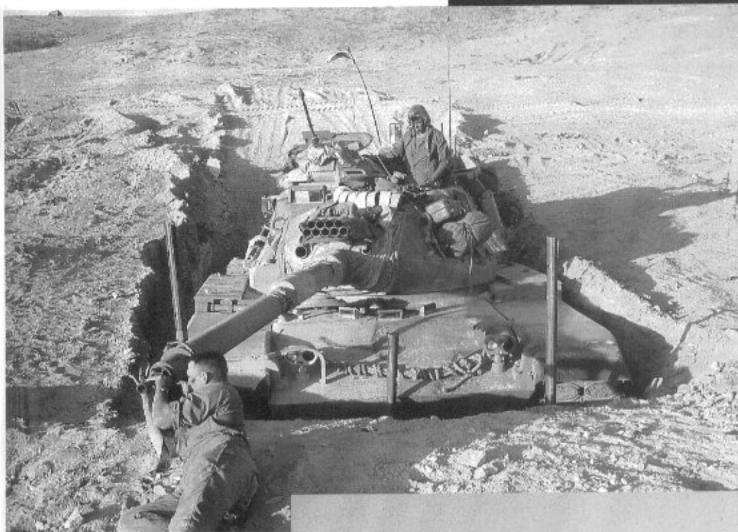
A tanker is bore-sighting his 105mm gun armed M60A3 tank. (Greg Stewart Photo)
