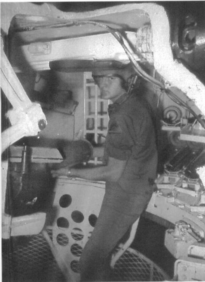
Two photos of the loader's position on an M30 turret trainer. The M30 is a training aid used to train personnel in the operation of the turret, the 105mm gun cannon, and the sighting and fire-control equipment of the M60 tank. The M30 trainer is a modified M60 tank turret mounted on a stand. The turret is provided with platforms and cut-out areas to allow the instructor to observe the trainee under actual operating conditions. It is powered from a rectifier power supply which replaces vehicle power. (U.S. Army Photos)
