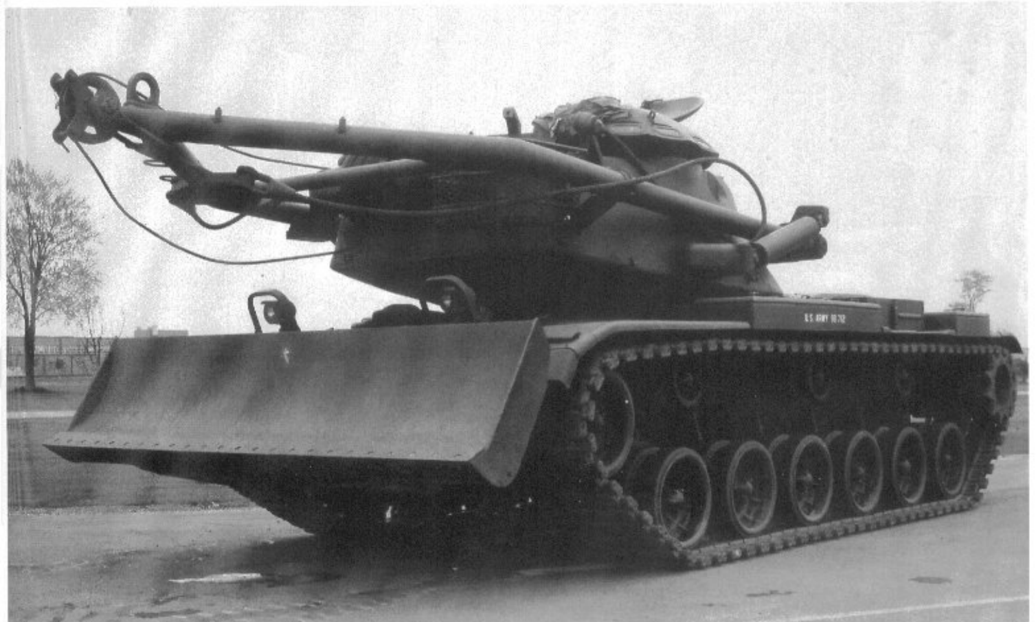
Equipped with a large "A" frame boom mounted on the turret of the CEV, the boom could lift almost nine tons. (U.S. Army Photo)
