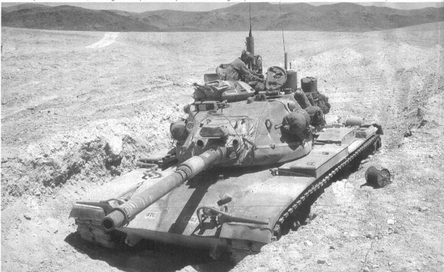
Another improvement to the M60A3TTS tank, one of the few that alters the outward appearance when compared to earlier models, is the addition of a thermal shroud on the main gun tube to aid in heat distribution. This shroud is mounted on the gun tube to minimize barrel distortion resulting from uneven heating that has, in the past, been a major cause of inaccuracy. (Greg Stewart Photo)
