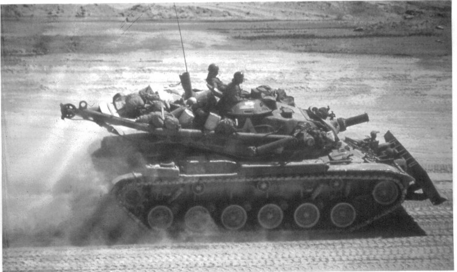
Overhead photo of an U.S. Army M728 Combat Engineer Vehicle with dozer blade raised and A-frame in travelling configuration, somewhere in Saudi Arabia. (U.S. Army Photo)
