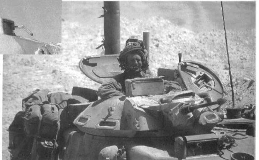
The cupola is a self-contained unit mounted and secured to the top of the turret. The cupola mounts the .50 cal. machine gun and contains the necessary controls to lay and fire the machine gun in azimuth (deflection) and elevation. (Greg Stewart Photos)
