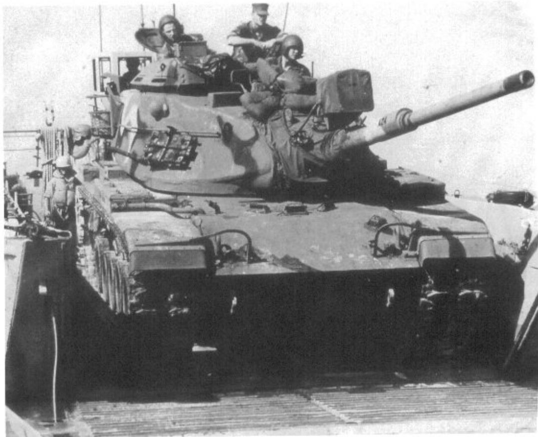
For combat operations from landing craft, the Marine Corps fitted their M60A1 tanks with fording kits. The vehicle could not be submerged completely under water, but with watertight snorkels fitted to the engine compartment, the M60 tank could wade ashore through very deep surf conditions, if needed. (U.S. Marine Corps Photos)
