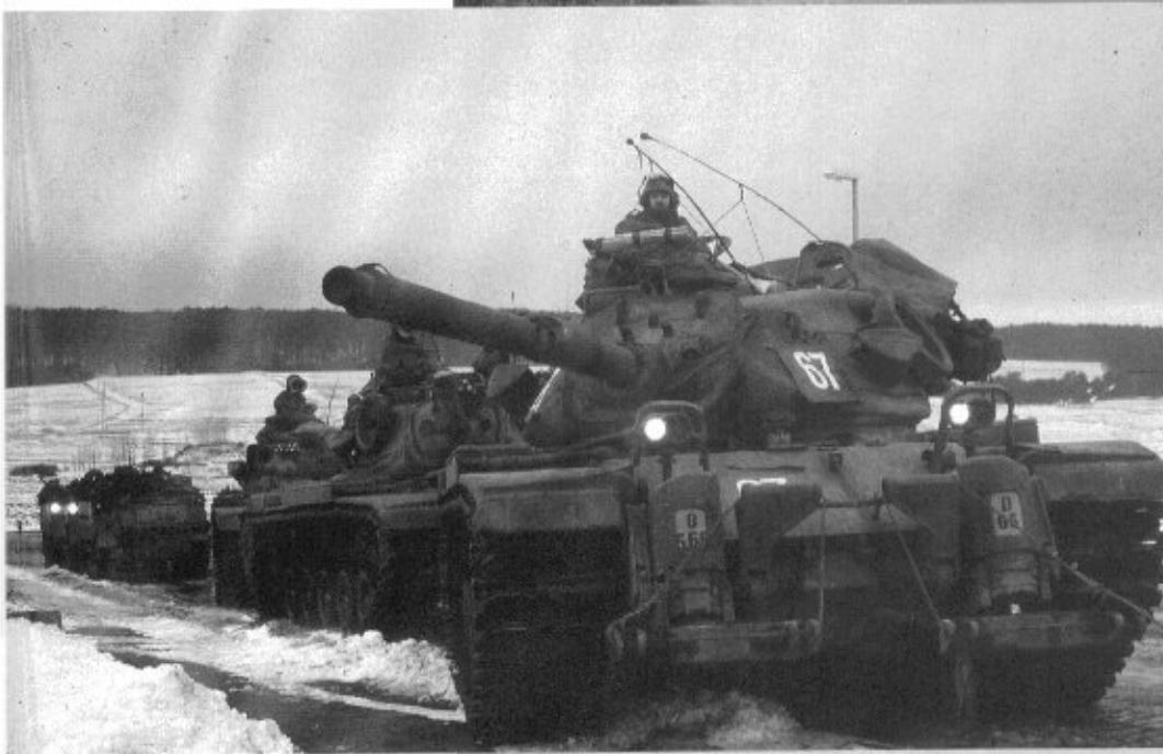
An M60A3 tank is seen here fitted with the M9 bulldozer kit, minus the bulldozer blade. You can clearly see the hydraulic supports needed to raise and lower the bulldozer blade. (Yves Debay Photo)
