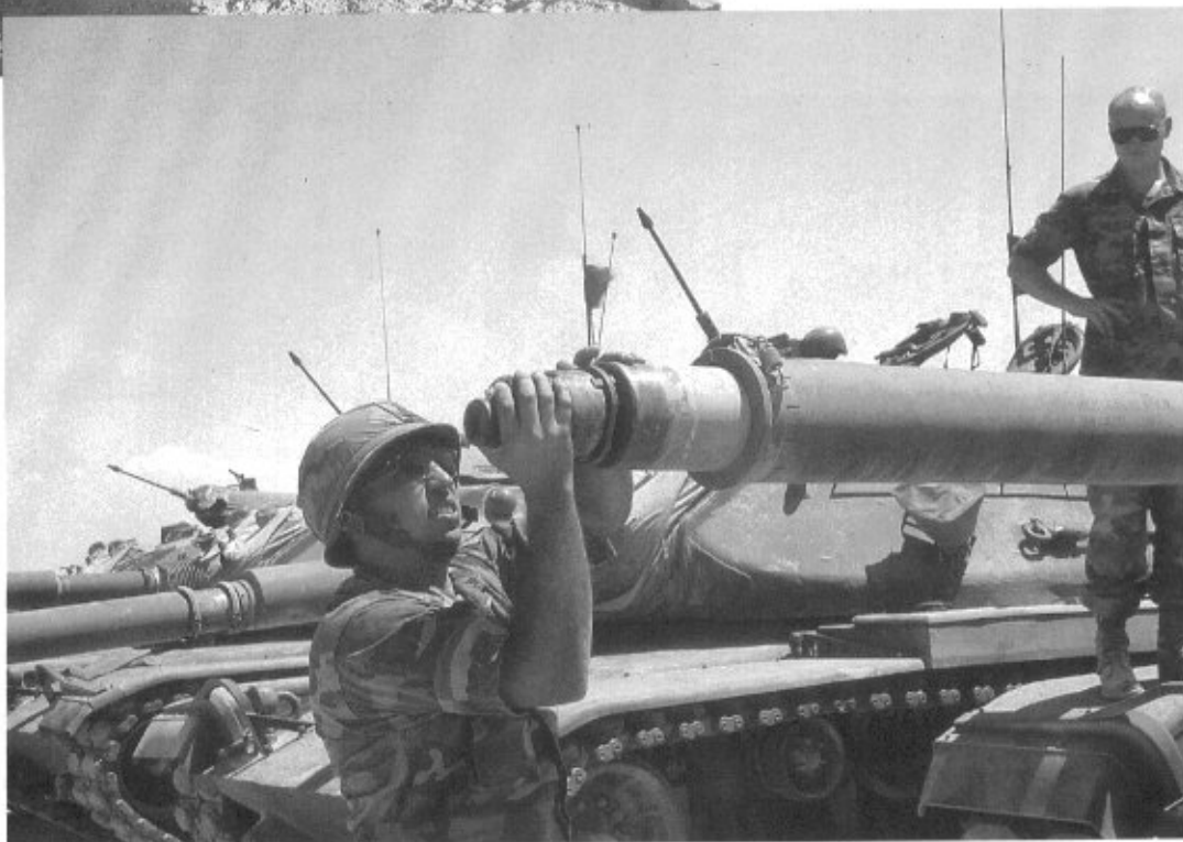
A 4th Infantry Division, 185th Armored Battalion tanker installs a boresighting device into the barrel of the main gun of an M60A3. (Greg Stewart Photo)
