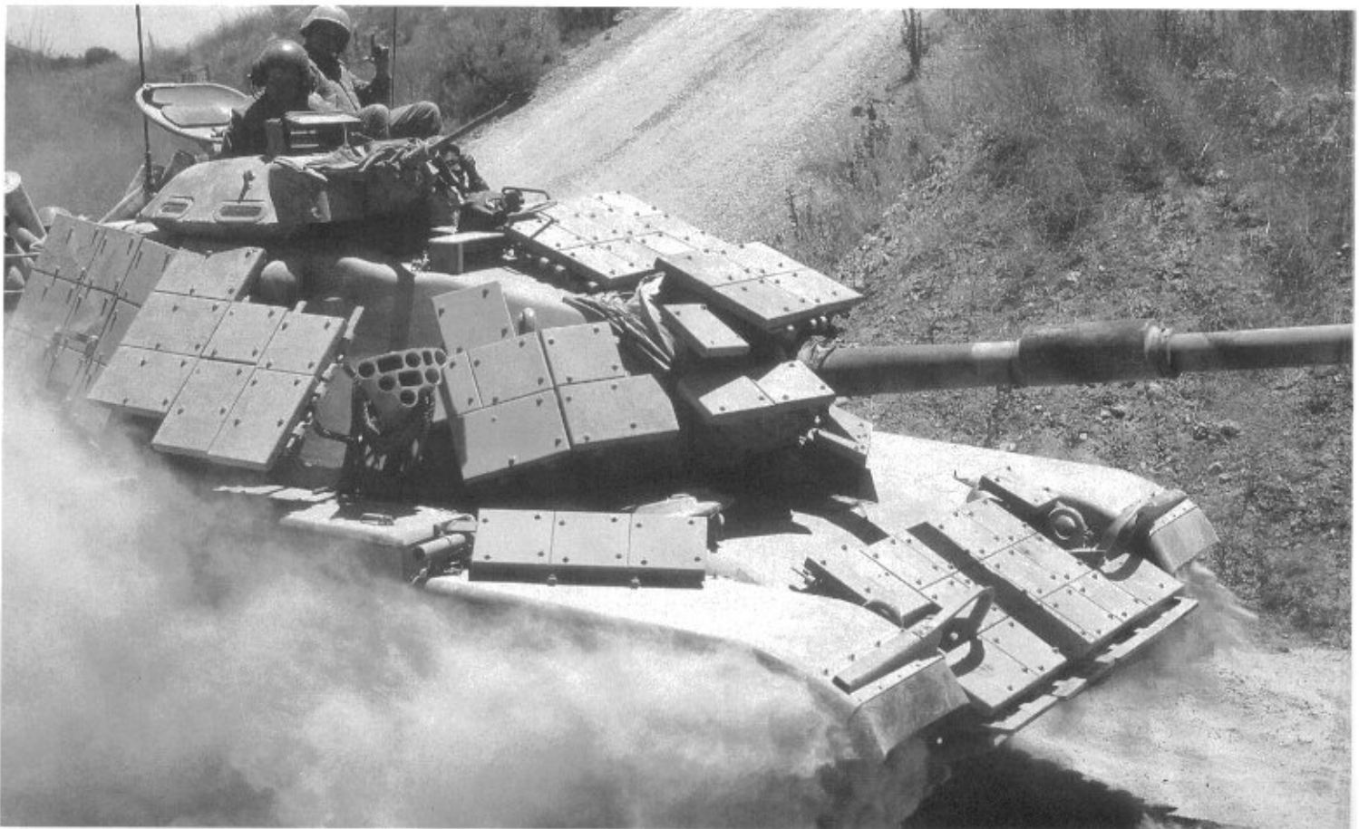
The reactive armor tiles are mounted to the exterior of the tank's hull and turret, and consists of 91 armor tiles (49 M1 tiles and 42 M2 tiles) which attach to mounting hardware using retaining clips and machine bolts. Some of the outside tow cables and brackets have had to be modified and/or relocated due to the installation of reactive armor. (Greg Stewart Photo)
