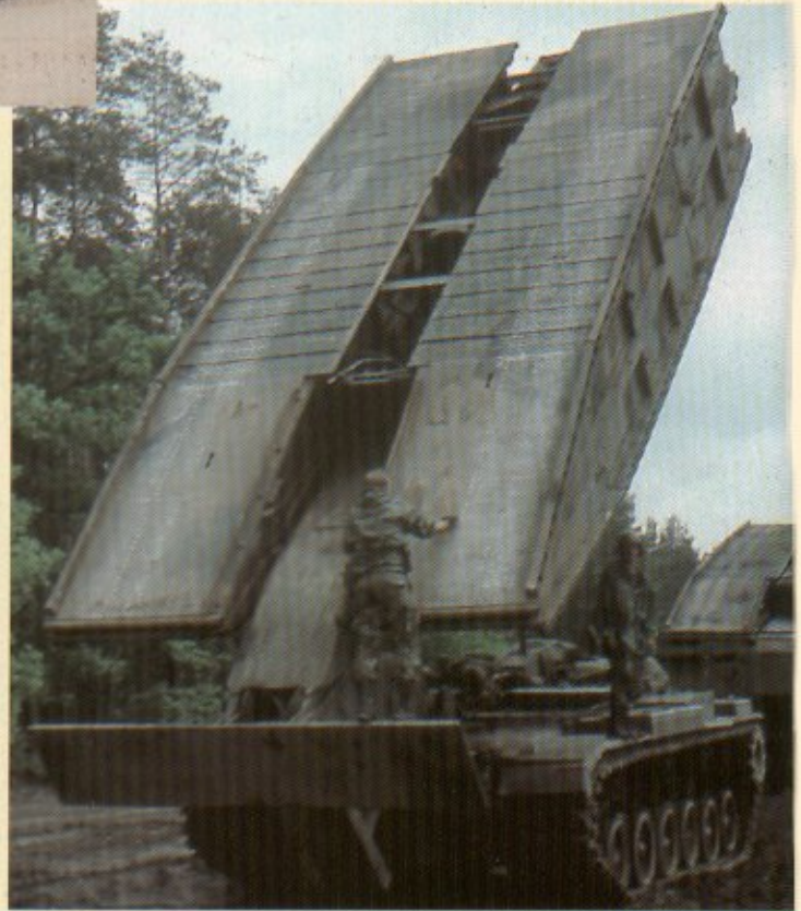
The M60 AVLB weights a little over 61 tons with a 60 foot bridge on board. There is also a 43 foot bridge that can be carried by this vehicle (Mike Green Photo)
