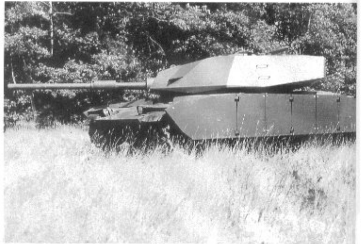
Teledyne Continental Motors, General Products Division, developed in 1981 as a private venture a high performance version of the M60 series tank. A standard M60A1 was fitted with a 1,200 hp diesel engine, four-speed hydromechanical transmission, a hydropneumatic suspension system, and an add-on armor package. (Teledyne Photo)
