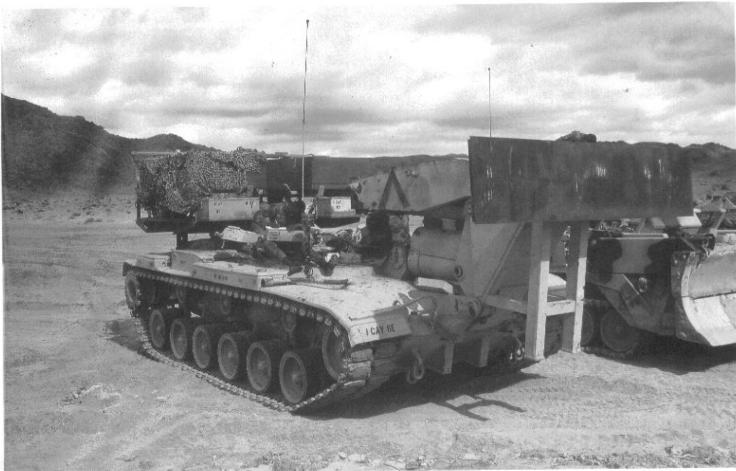
Some M60 AVLB have been converted to Armored Vehicle Launched MICLICs (AVLM) to carry two Mine Clearing Line Charge (MICLIC) systems. The MICLIC is capable of sending a line charge into a minefield and upon detonation clearing a 100 by 8 meter path. (Greg Stewart Photos)
