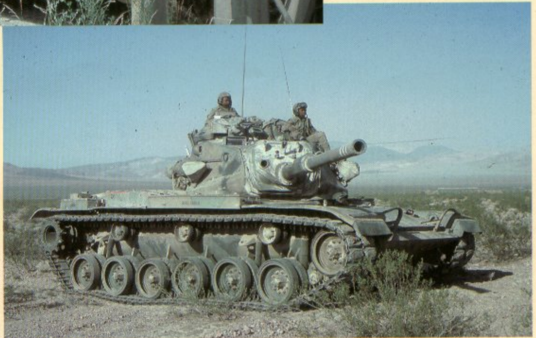
The armament consists of a 105mm gun cannon mounted in a combination gun mount M116, or M140, a coaxially mounted 7.62 machine gun mounted on the combination gun mount, a .50 cal. machine gun mounted in the commander's cupola M19. The 105mm gun cannon consists of a gun tube, evacuator chamber group, breech operating group, breech ring group, and breechblock group. (Greg Stewart Photo)
