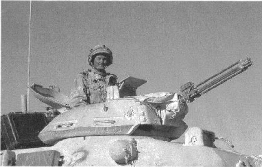
The cupola is a self-contained unit mounted and secured to the top of the turret. The cupola mounts the .50 cal. machine gun and contains the necessary controls to lay and fire the machine gun in azimuth (deflection) and elevation. (Greg Stewart Photos)
