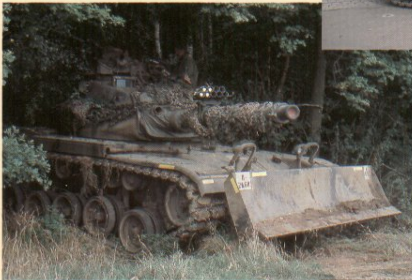
The value of a tank mounted bulldozer for clearing obstacles or debris under fire was clearly demonstrated during WWII. During the postwar period bulldozer kits were designed to be fitted to the entire series of Patton tanks, from M46 thru M60A3. Pictured is an U.S. Army M60A3, with a bulldozer blade mounted, hiding in a wooded cove in West Germany. (Yves Debay Photo)
