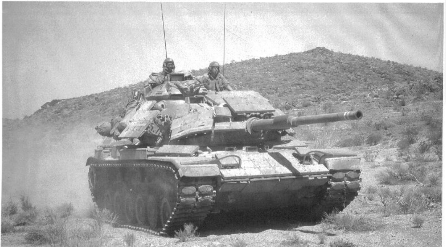
A total of 91 armor tiles are required for the basic M60A1 (RISE/PASSIVE) tank. Forty-nine M1 tiles, which are 11.5 inches by 11.5 inches x 2 inches in size, and forty-two M2 tiles, which are 11.5 inches x 17.5 inches x 2 inches in size. Dummy (inert) tiles are used on currently fielded M60A1 Marine Corps tanks. The real tiles are stored until needed in a wartime environment. Marine Corps tanks stored on Marine Prepositioned Ships (MPS) are outfitted with live tiles. Since the dummy tiles weight less than the real tiles, weighted tiles have to be left on the turret main gun mantel to keep the 105mm main gun in balance. (Greg Stewart Photo)
