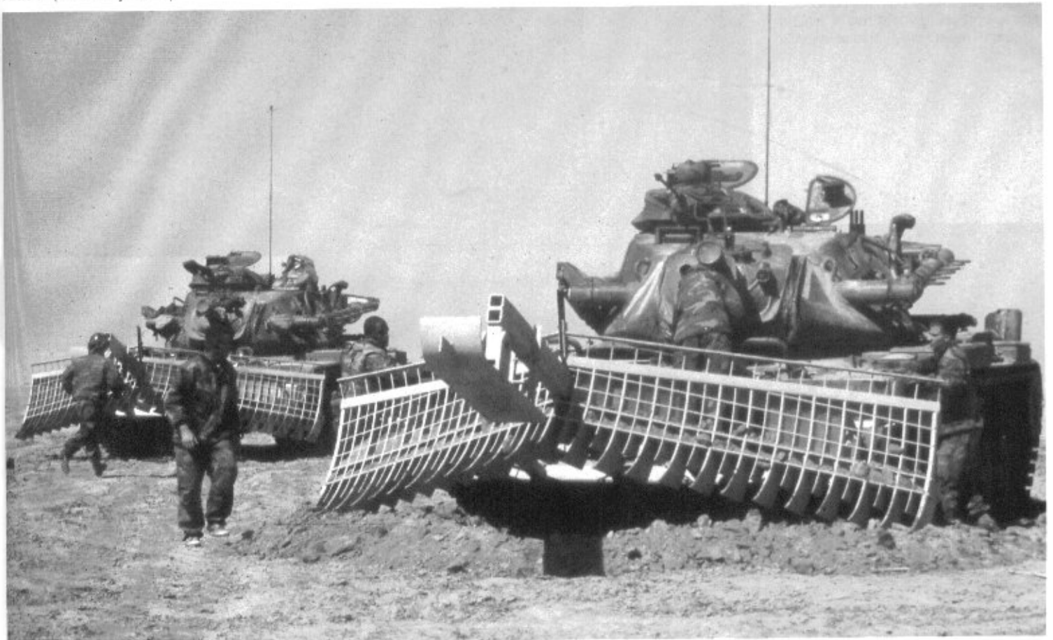
The 24th Mechanized Infantry Division deployed a number of M728 Combat Engineer Vehicles to Saudi Arabia in 1991. The vehicles were mounted a brand new mine clearing rake. Created for sand or loose soil, the 12-inch rake was used by both Army and Marine Corps combat engineers in Saudi Arabia to breach a 180-inch path through Iraqi minefields. This is wide enough to allow an M1A1 to pass. (DoD)
