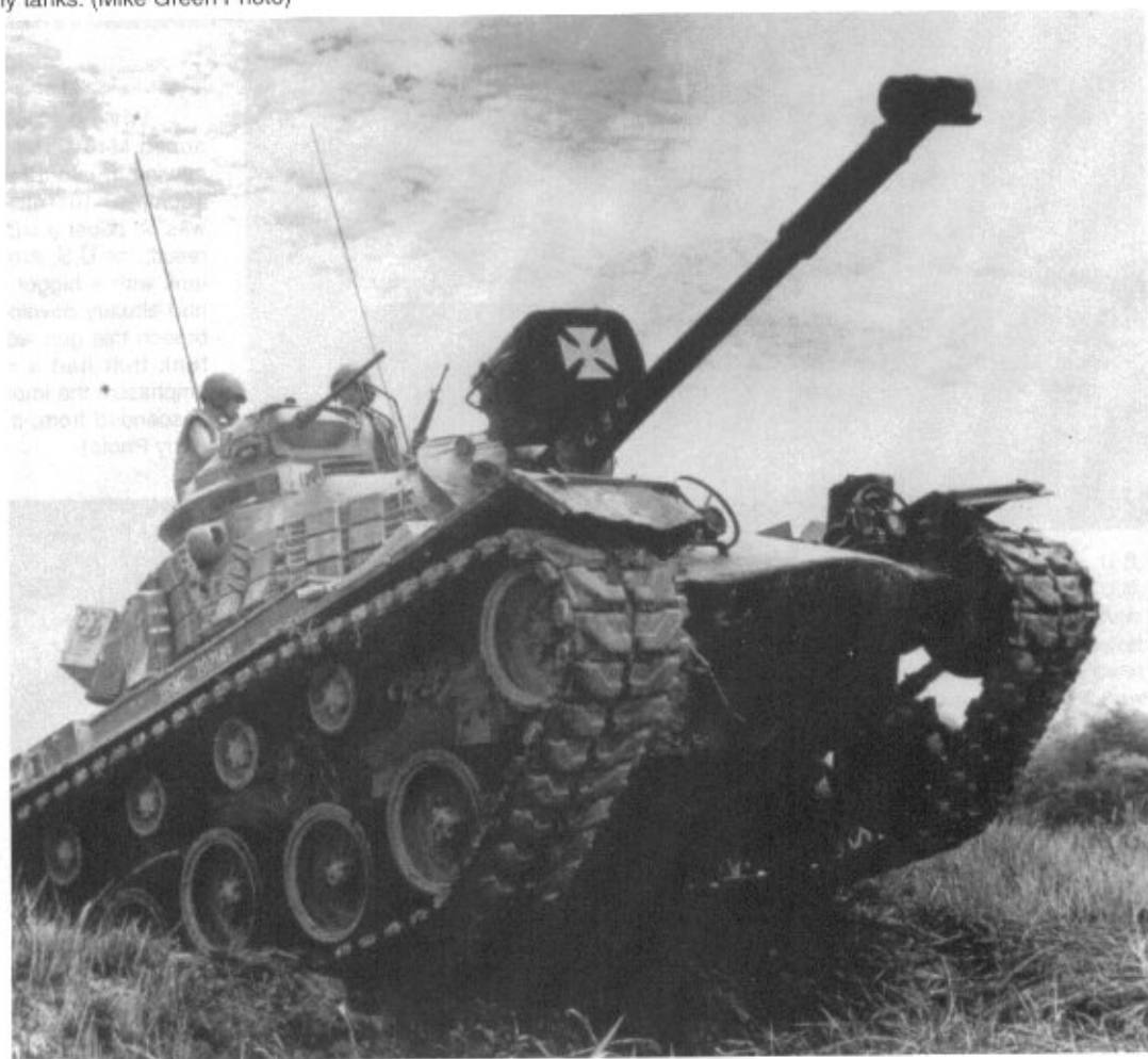
In 1953, the M48 90mm gun armed tank was introduced. This tank had a boat-shaped hull and hemispherical turret to provide better ballistic protection against antitank projectiles. There were improved ammunition storage methods and a more efficient fire control system. The M48 had a crew of four in contrast to the five found in earlier U.S. Army tanks. (Mike Green Photo)
