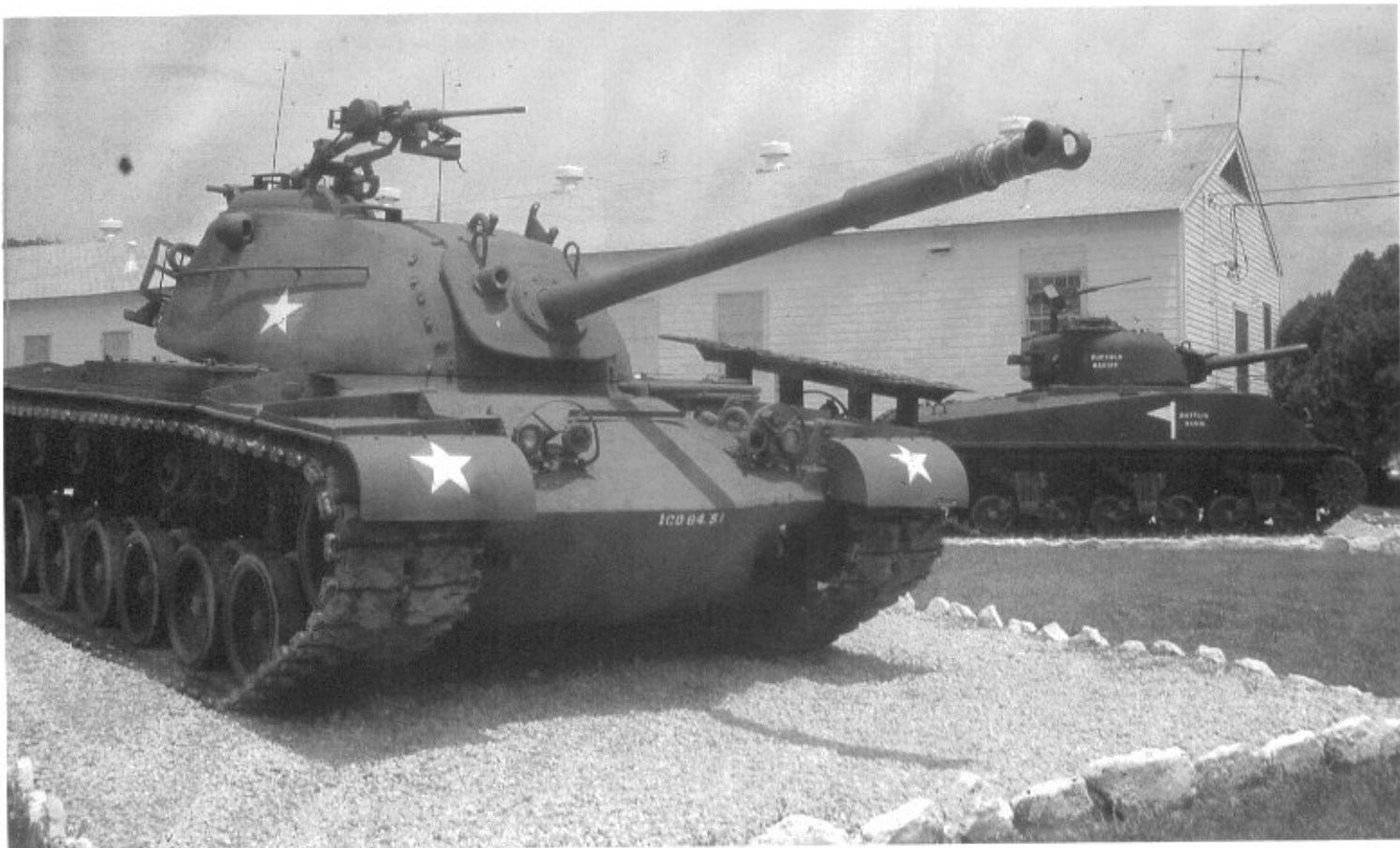
In 1953, the M48 90mm gun armed tank was introduced. This tank had a boat-shaped hull and hemispherical turret to provide better ballistic protection against antitank projectiles. There were improved ammunition storage methods and a more efficient fire control system. The M48 had a crew of four in contrast to the five found in earlier U.S. Army tanks. (Mike Green Photo)
