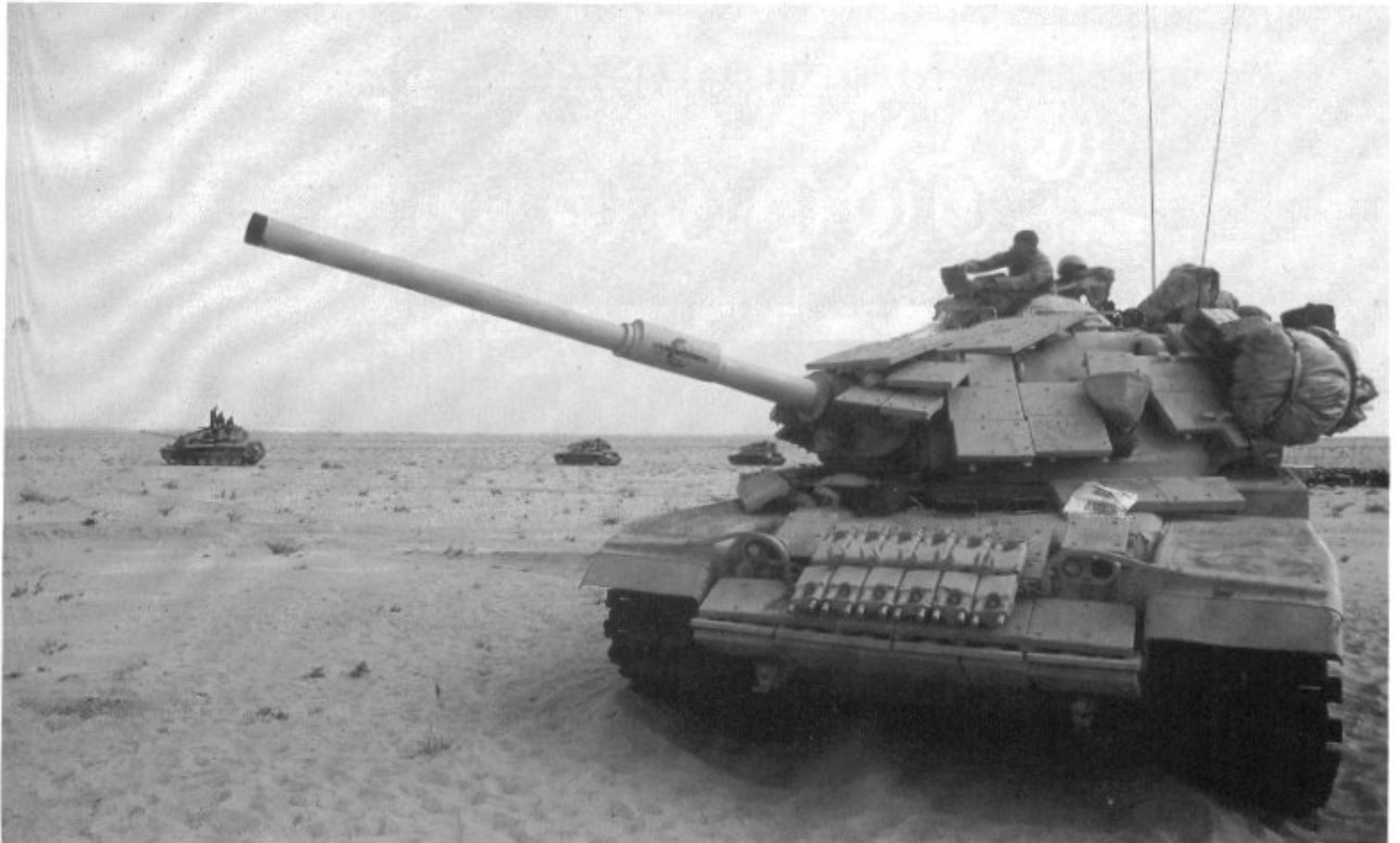
"American Express" M60A1 with reactive armor tiles during a training exercise in Saudi Arabia prior to Operation Desert Storm. Note the spare tracks and the amount of personal gear hanging on the side of the turret. (Yves Debay Photo)
