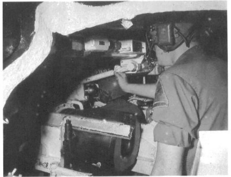
Two photos of the loader's position on an M30 turret trainer. The M30 is a training aid used to train personnel in the operation of the turret, the 105mm gun cannon, and the sighting and fire-control equipment of the M60 tank. The M30 trainer is a modified M60 tank turret mounted on a stand. The turret is provided with platforms and cut-out areas to allow the instructor to observe the trainee under actual operating conditions. It is powered from a rectifier power supply which replaces vehicle power. (U.S. Army Photos)
