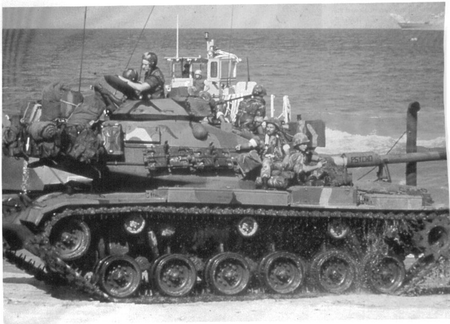
For combat operations from landing craft, the Marine Corps fitted their M60A1 tanks with fording kits. The vehicle could not be submerged completely under water, but with watertight snorkels fitted to the engine compartment, the M60 tank could wade ashore through very deep surf conditions, if needed. (U.S. Marine Corps Photos)
