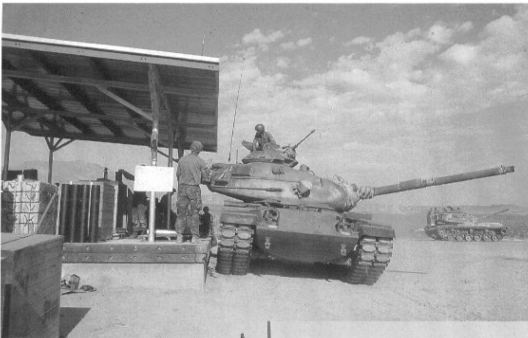
An 185th Armor M60A3 being loaded with 105mm main gun ammunition on a livefire range at the National Training Center. (Greg Stewart Photo)
