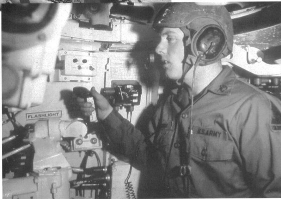
Tank commander of an M60A1 inside the turret with his right hand on the turret controls. (U.S. Army Photo)
