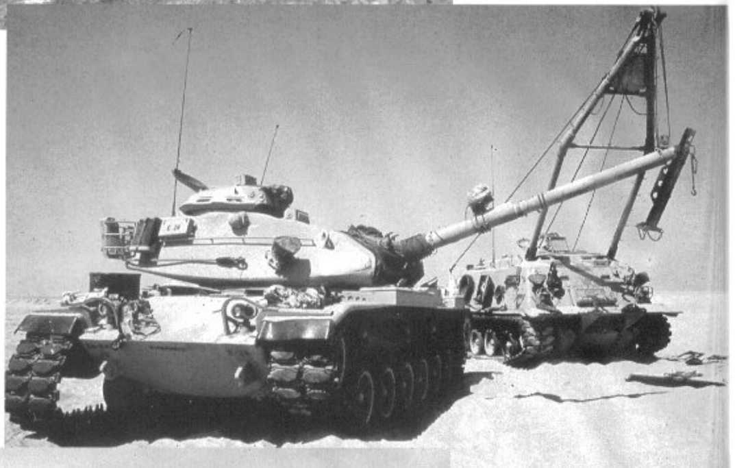
This M60A3 lost its tracks and is being retrieved by an M88. (U.S. Army Photo)
