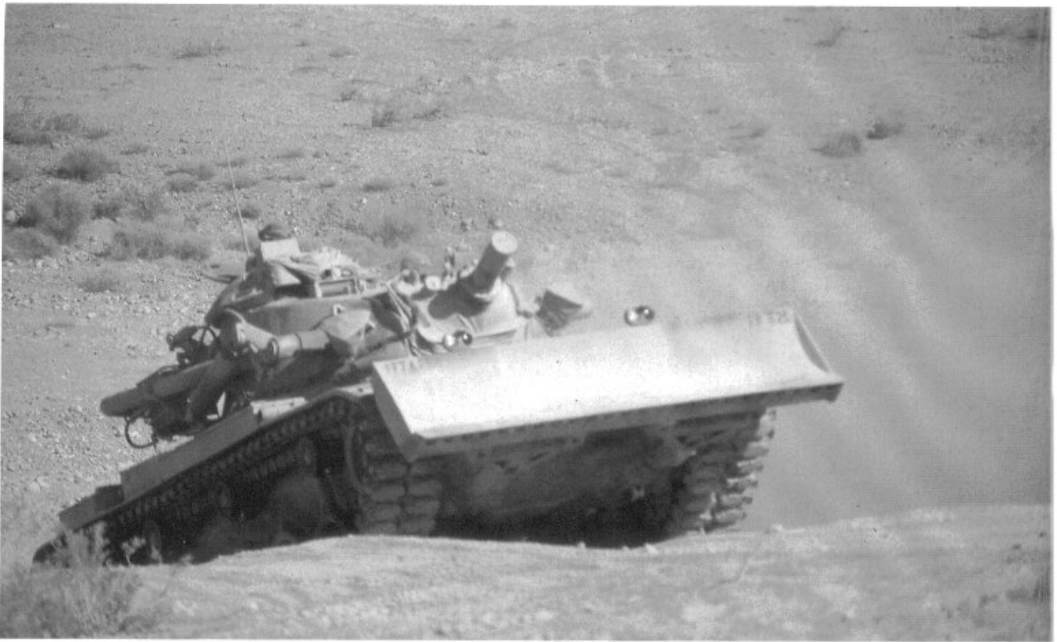
The CEV was also fitted with a M9 bulldozer blade on the front of the vehicle. The CEV's bulldozer blade is wider than its hull, hence it can excavate a full-width tank position, suitable for both M60 and M1 tanks, in a single pass. (Greg Stewart Photo)
