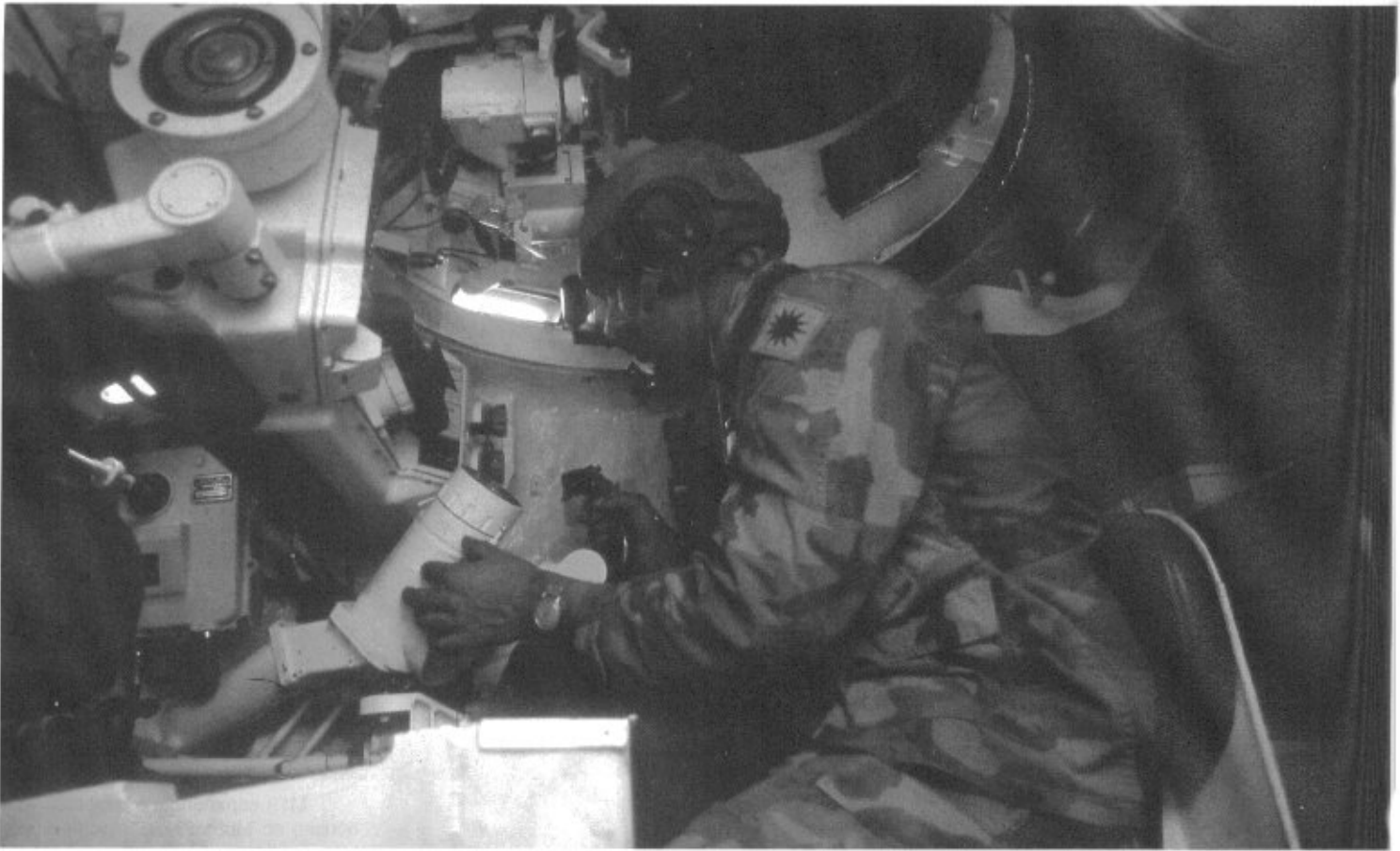
The tank commander of an M60A3 tank looking into his thermal viewer. (Mike Green Photo)
