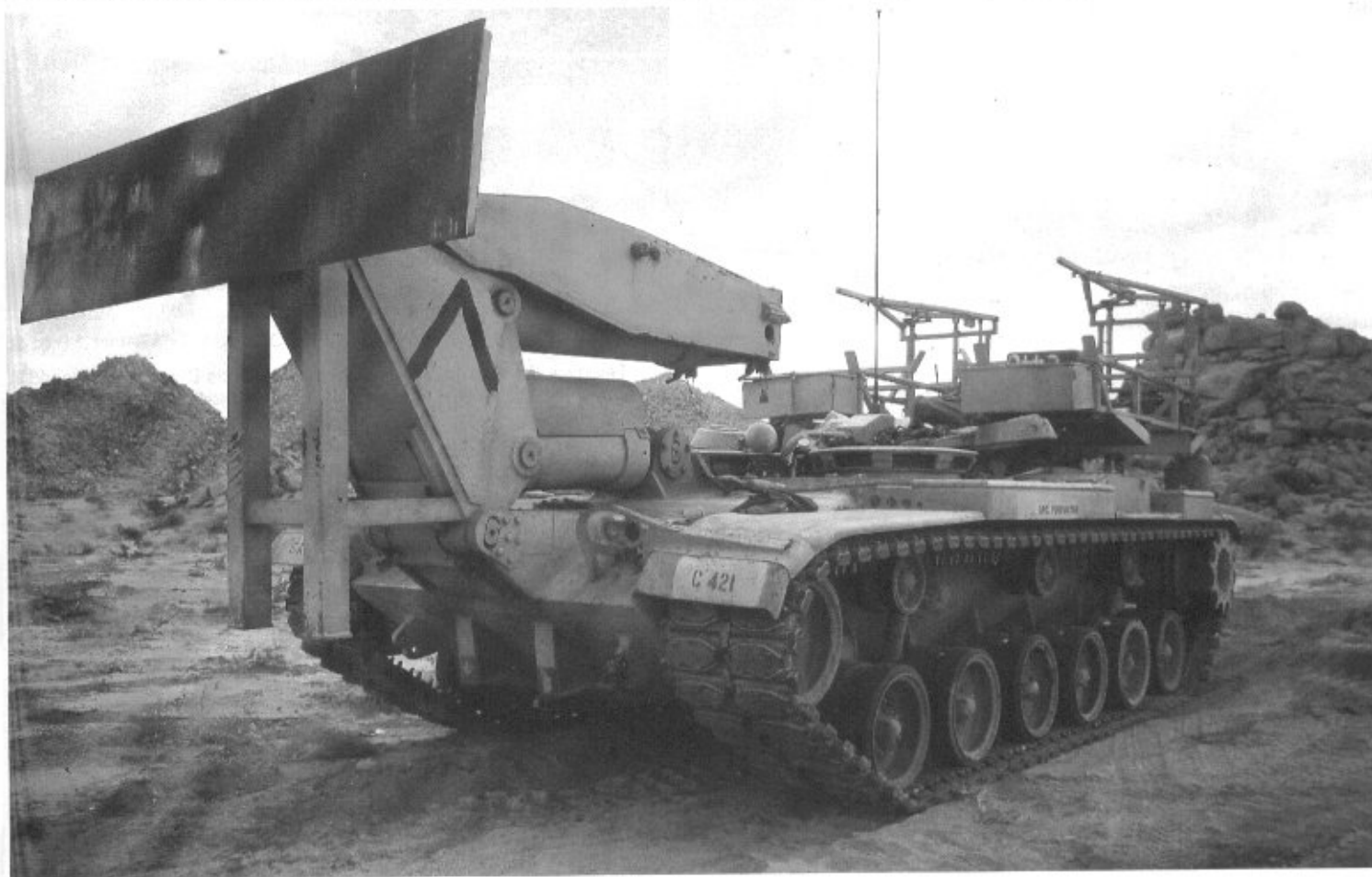
Some M60 AVLB have been converted to Armored Vehicle Launched MICLICs (AVLM) to carry two Mine Clearing Line Charge (MICLIC) systems. The MICLIC is capable of sending a line charge into a minefield and upon detonation clearing a 100 by 8 meter path. (Greg Stewart Photos)
