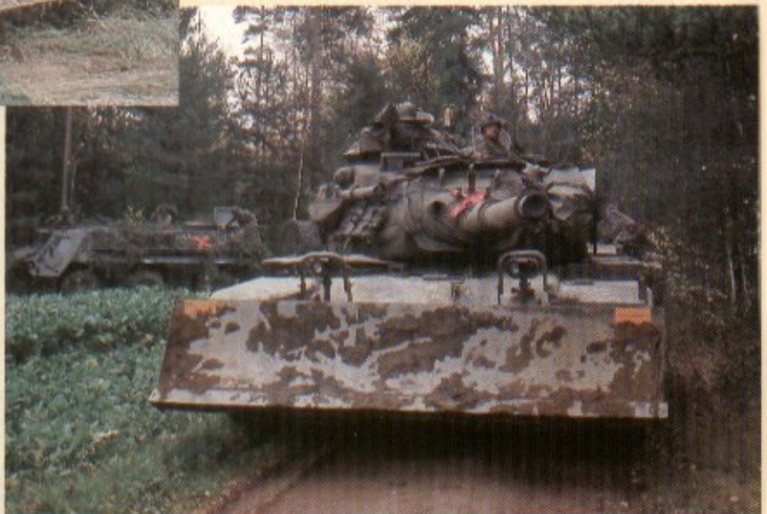
Pictured is a head-on photo of an M60A3 tank in West Germany during REFORGER 1988, mounting a M9 bulldozer kit. The blade is raised for traveling mode. (Yves Debay Photo)
