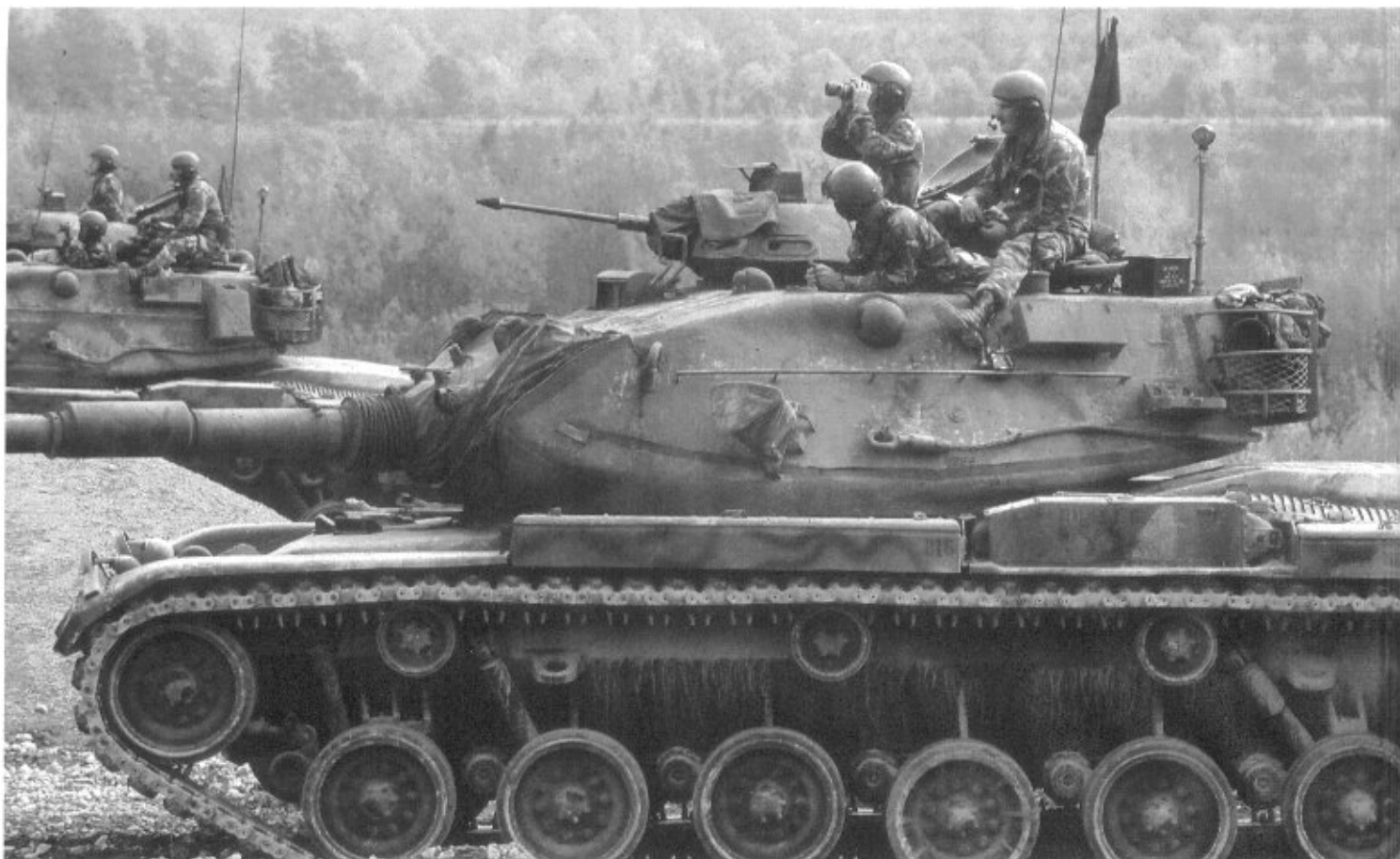
The M60A3TTS tank also has been equipped with a wind drift sensor, mounted on the rear of the turret that automatically inputs the ballistic computer with wind speed and direction, enabling the computer to compensate the main gun's point of aim. (Fort Knox Public Affairs Office Photo)
