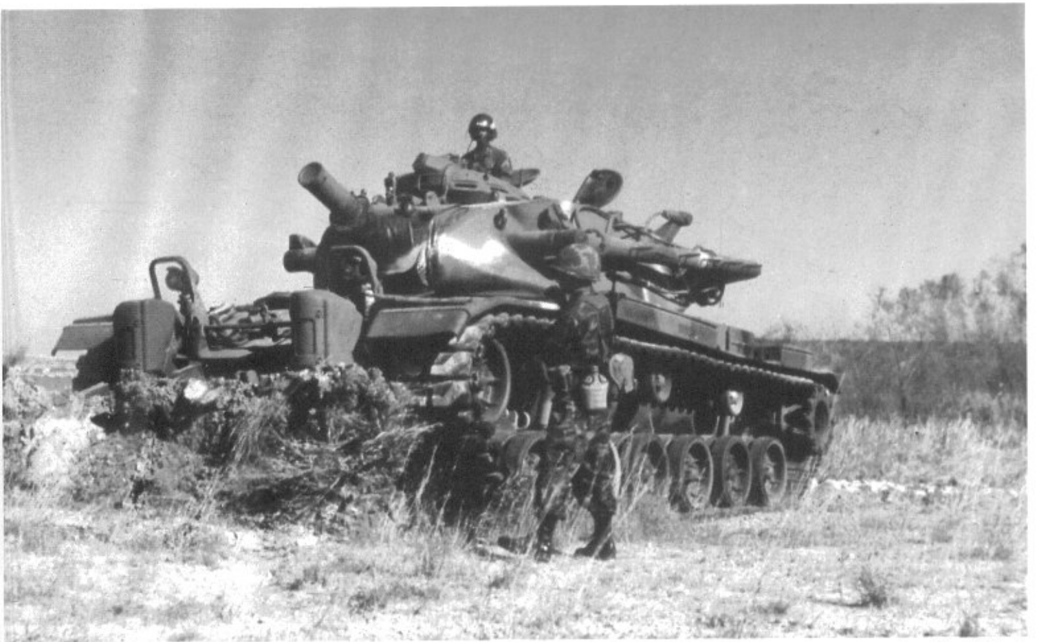
The M728 Combat Engineer Vehicle (CEV), which was issued to U.S. Army units beginning in 1966, was a specially designed version of the M60 tank produced for use by Army combat engineering units. Intended to clear any type of obstacle that may slow down the advance of other armored vehicles such as tanks and armored personnel carriers, the CEV could remove roadblocks or damaged vehicles under combat conditions. (U.S. Army Photo)
