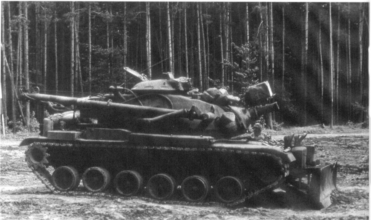
Located in the rear of the CEV turret is a 25,000 pound capacity winch for towing other vehicles out of difficult terrain. To destroy enemy pillboxes or bunkers, the CEV was fitted with a short-barrelled 165mm gun based on a British-made L9A1 cannons. Because of the size of the 165mm round, only thirty rounds can be carried by the CEV. Combat loaded the CEV weights 57.5 tons. Over 243 CEVs were built between 1966-1972. A few even saw service in the Vietnam War. (Mike Green Photo)
