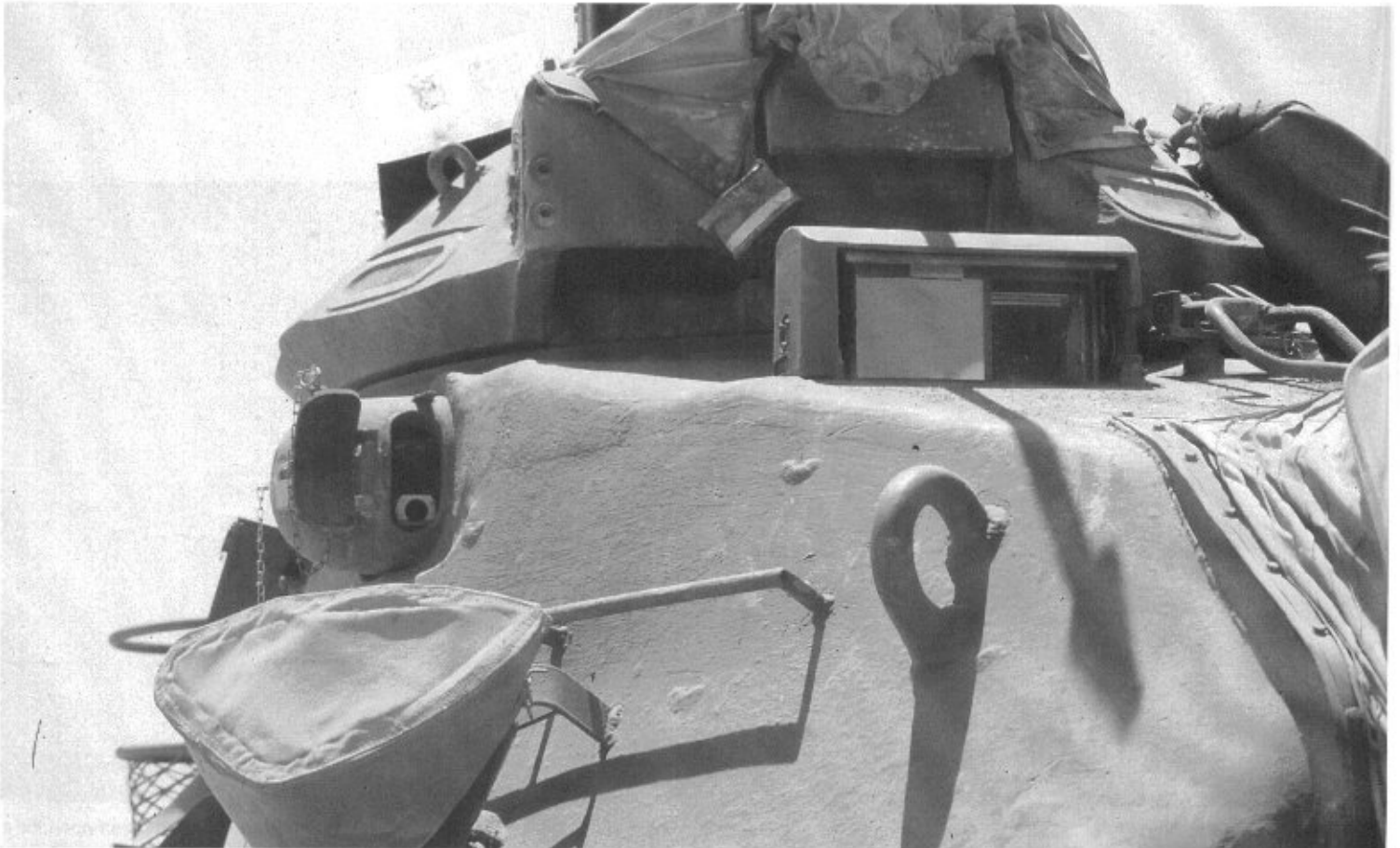
Detail of right side of M60A3 turret showing (TTS) Tank Thermal Sight and rangefinder with armored cover in open position. (Greg Stewart Photo)
