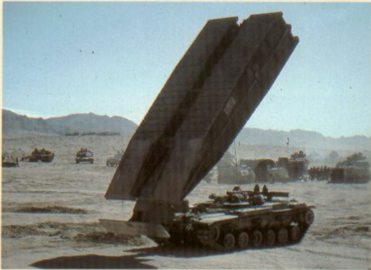
A 155th Armored Brigade M60 AVLB recovers a bridge span. The span can be connected at either end, allowing it to be recovered after the M60 AVLB passes over it. (Greg Stewart Photo)
