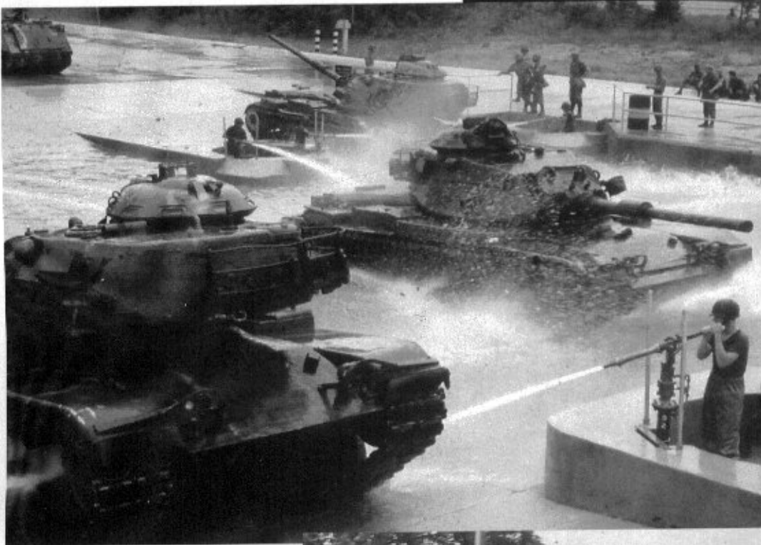
M60A1 tanks being cleaned with high-pressure water jets, the only way to get the mud, dust and dirt off that cakes itself on to the tanks during training. (U.S. Army Photo)
