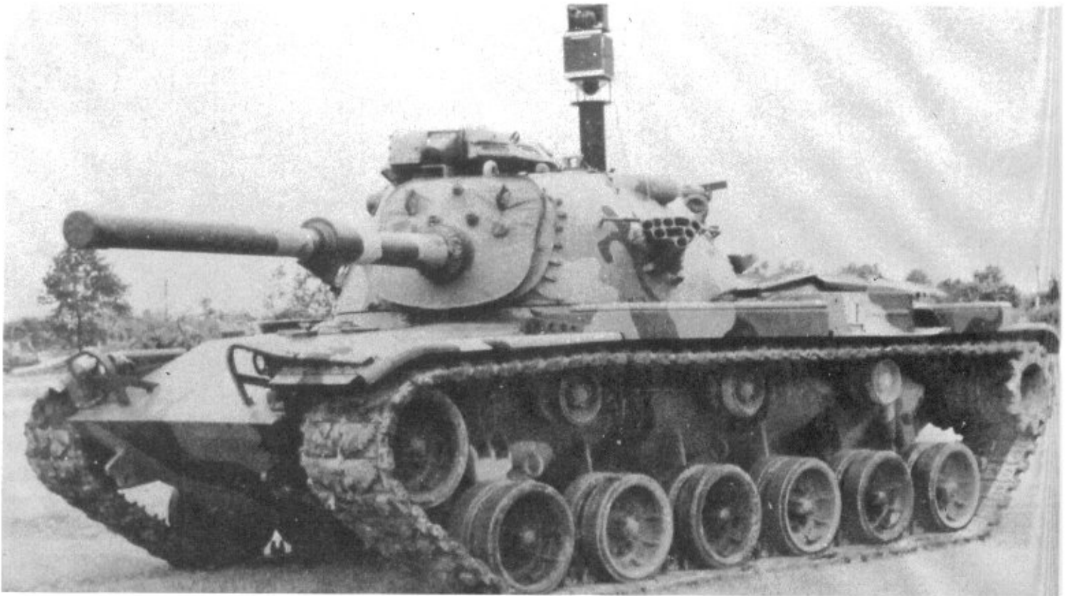
For test purposes, the U.S. Army attached a "breadboard automatic defense system" to an early model M60 tank. The system was designed to detect anti-tank missiles and to launch smoke grenades or thermoflares as countermeasure. (U.S. Army Photo)
