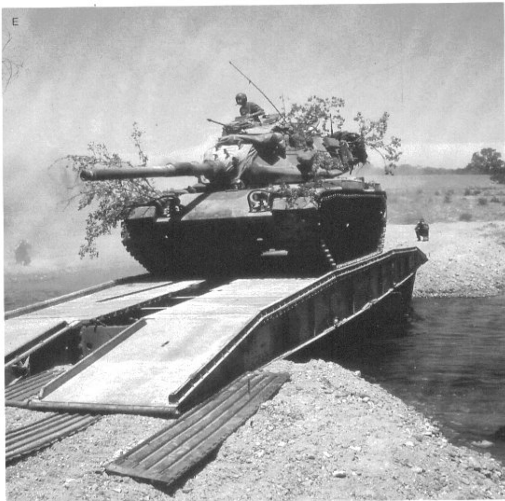
Under the best conditions it should only take two minutes to lower the bridge on the M60 AVLB and about ten minutes to recover it. (Mike Green Photos)
